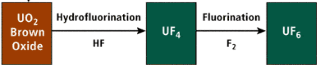
Process of turning uranium oxide (U 3 O 8 ) to uranium hexafluoride (UF 6 )
