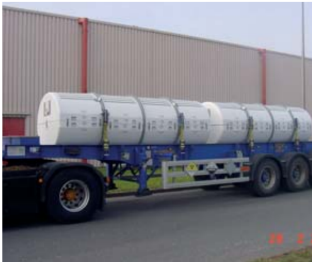
48Y Cylinder with outer protection
