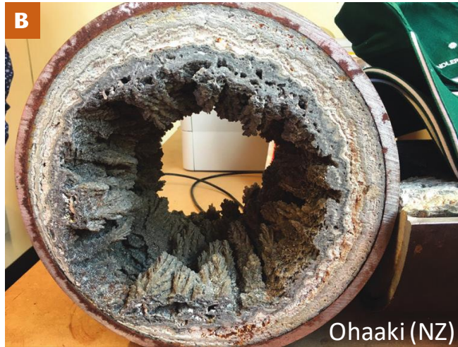
1. Mechanical extraction of mineral scales
