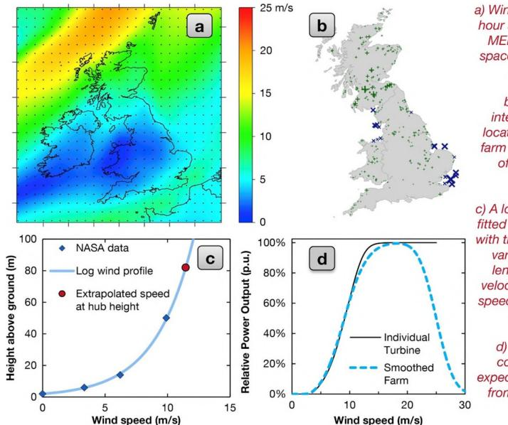
a) Wind speeds for each hour are acquired from MERRA's regularlyspaced grid (shown as black dots).
