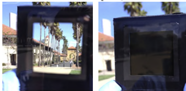
Solar modulation via tunable absorption (Reversible reactions, \text{VO}_2 , nanoparticles, etc.)
