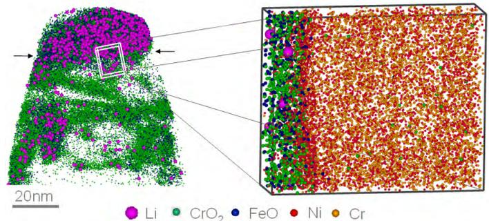
Oxidation of stainless steel in contact with reactor coolant
